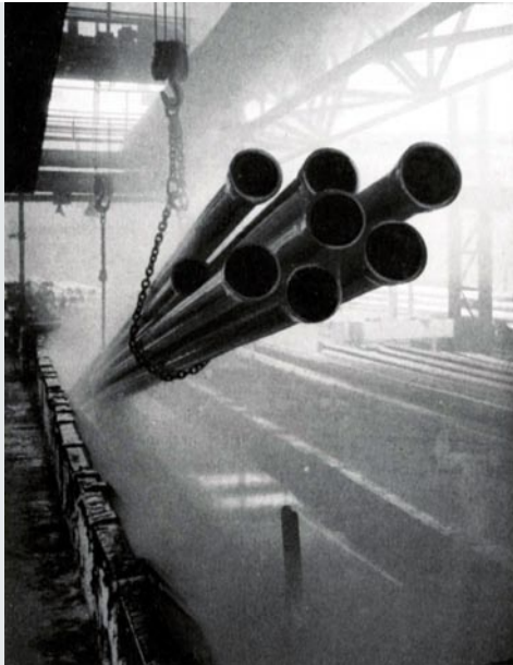
FIG. 9: Submerging steel piping in a bitumen bath
