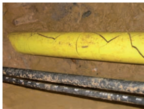
Fig. 3: Brittle fracture in an extruded polyethylene coating
