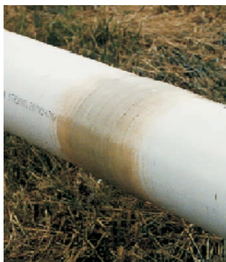
Fig. 5: Field joint coating of polypropylene coated pipes with an additional FRP system
